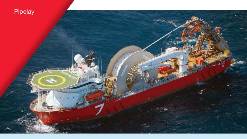
The Seven Navica is capable of installing both rigid and flexible products in water depths of up to 2,000m, with a top tension capacity of 205t.
