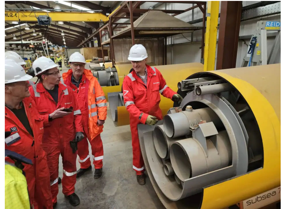
A pipeline bundle cross section at Wick
