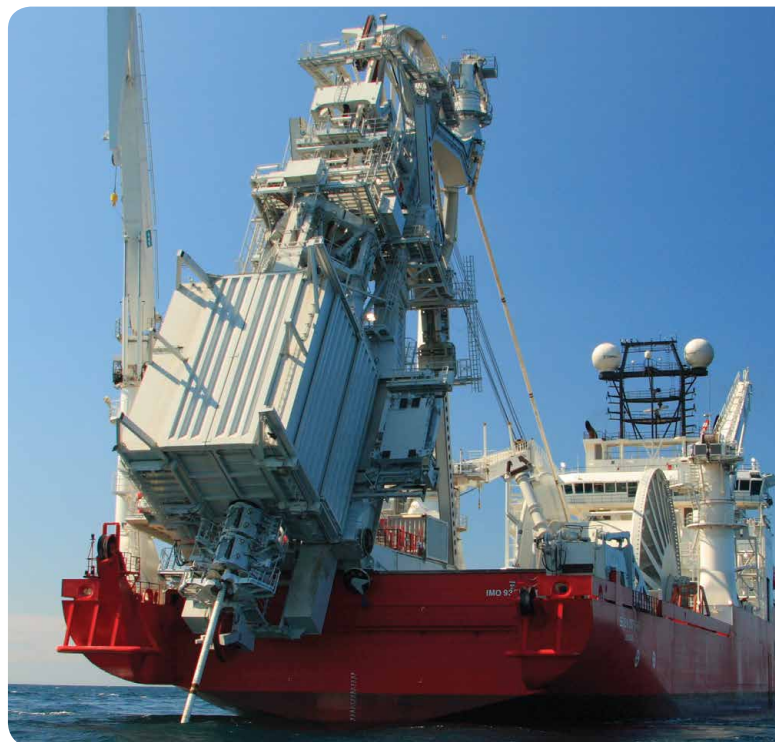
Subsea 7's reel-lay vessel Seven Oceans laying pipe
