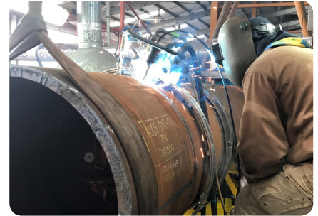
Welding procedure qualification testing being conducted at Serimax facility in Johor Baru, Malaysia
