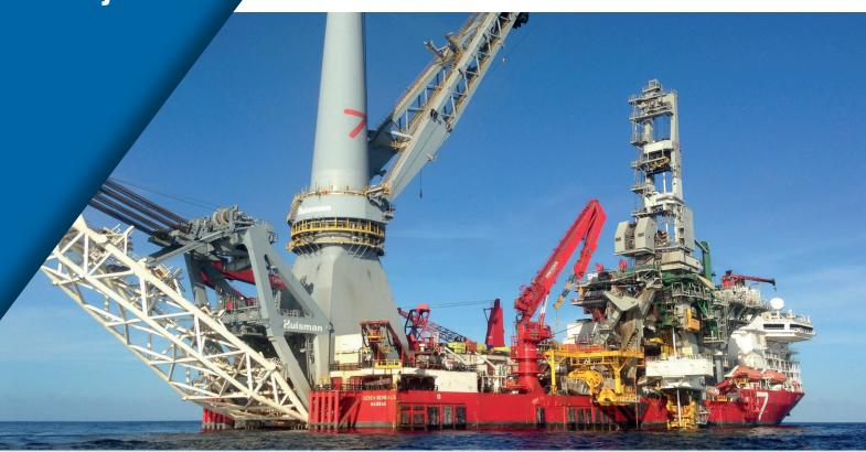
The Heidelberg Development is located in the southern Green Canyon block of the Gulf of Mexico. The field includes two drill centers tied back to a truss Spar via 8-inch flowlines and Steel Catenary Risers. The processed oil and gas is then exported via two 16-inch export lines.
