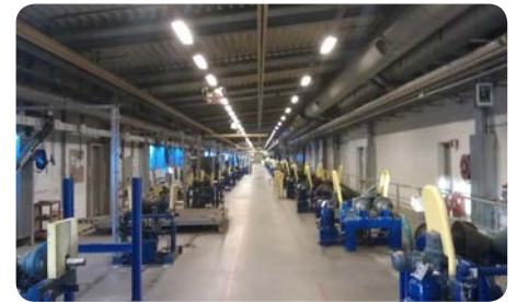
On the right the double joint line, on the left the main line fabrication line
