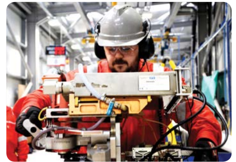
Non Destructive Examination tests weld quality
