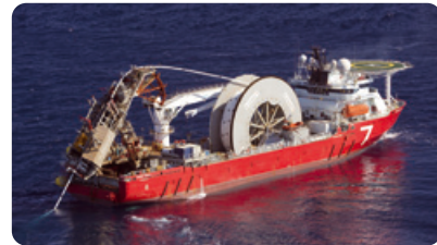
Seven Navica pipelay vessel
