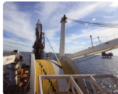
Seven Oceans laying pipe
