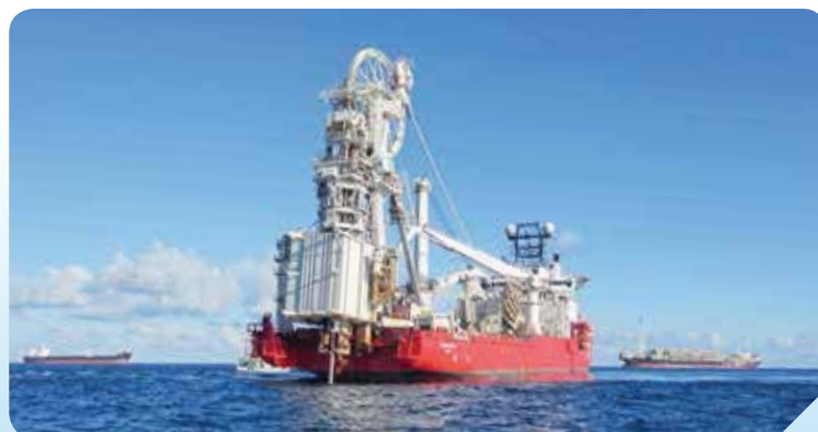
Seven Oceans J-laying BuBi ® corrosion-resistant pipe on the Guará-Lula NE project, Brazil
