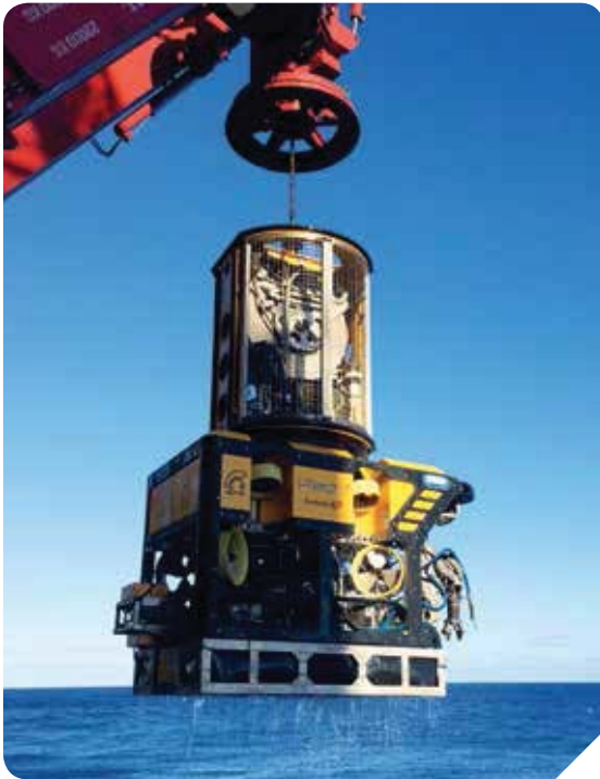
The new-generation i-Tech Centurion SP2 Remotely Operated Vehicle (ROV) is smaller and lighter than other units
